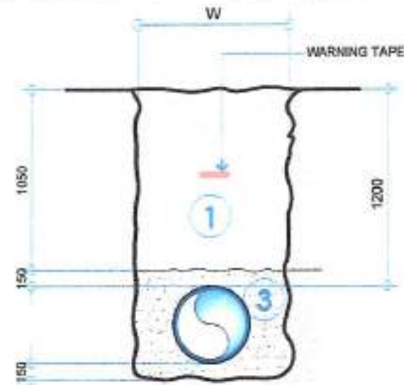
IN ROCK OR WHEN ORDERED BY ENGINEER
