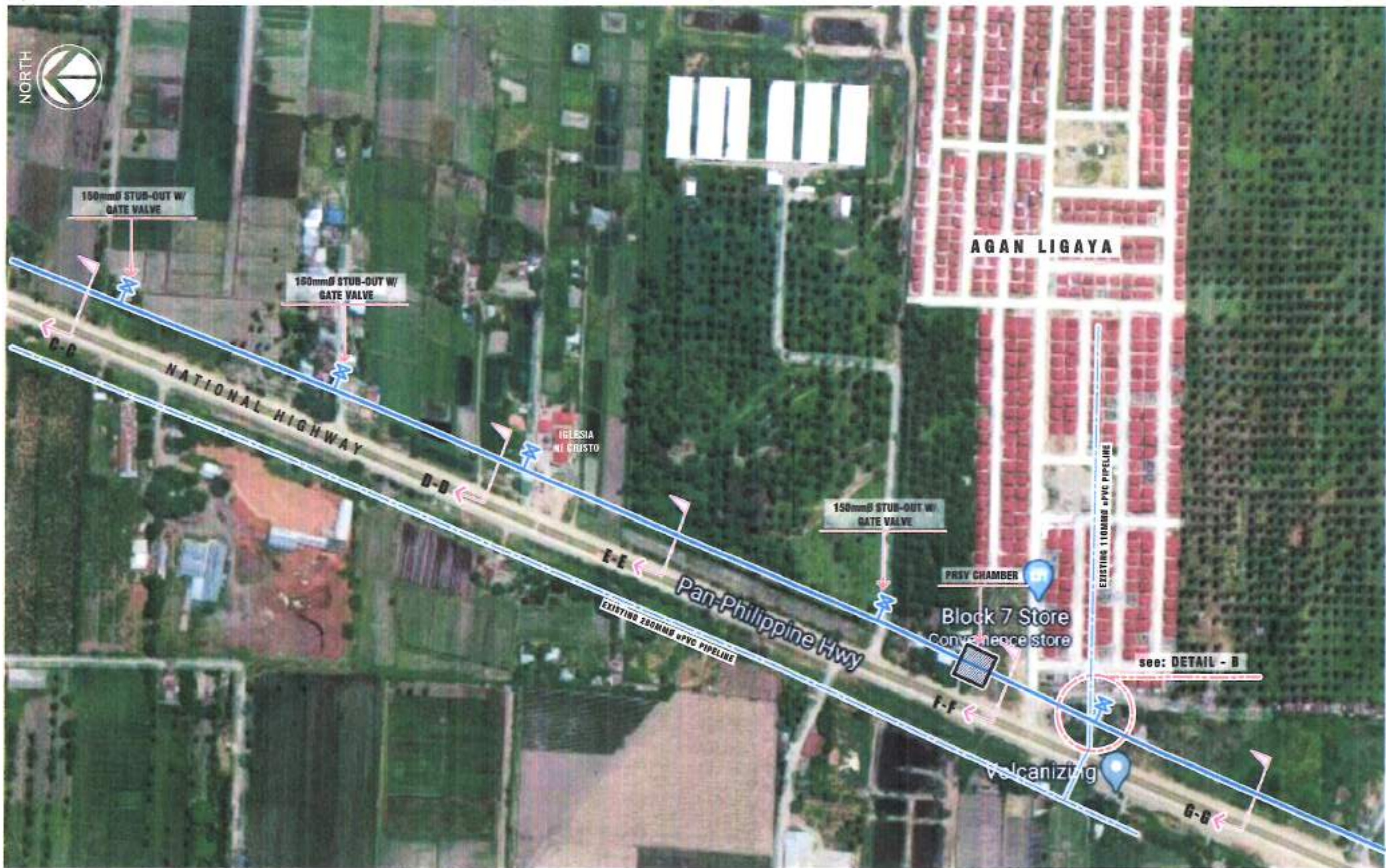
PIPE DISTRIBUTION LAYOUT SCALE: NTS
