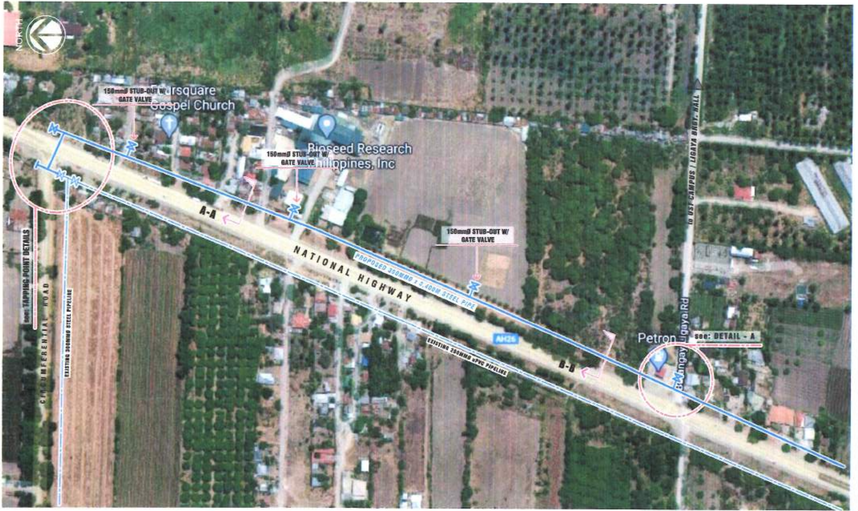
PIPE DISTRIBUTION LAYOUT SCALE: _____ N T S
