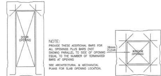
TYP. EXTERIOR WINDOW & DOOR OPENING
