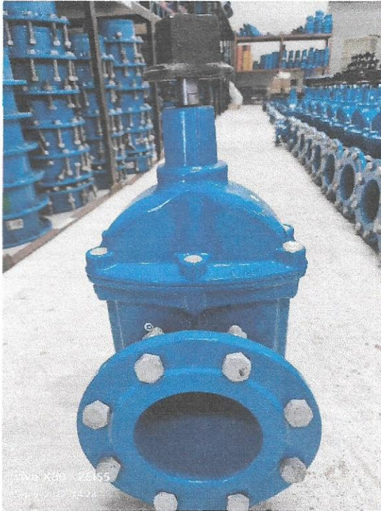
D.I. GATE VALVE 150MM F/F (WITH HOT DIP GALVANIZED BOLTS AND NUTS: PN 16)
